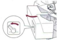
Remove free arm cover by swinging the extension table out with the lever in locked position. The free arm cover will stay attached to the extension table.
